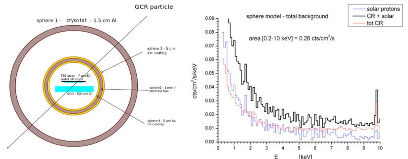
We initially prepared a simple geometrical model sphere model where we assumed a simplified geometry composed by 4 concentric spheres. This is a standard approach, often used in background simulations for space applications (H.Murakami, 2006). Simulations on the sphere model has been used to check the right response of the simulators, requiring low time machine computation, and has been run on a PC with standard performances.
