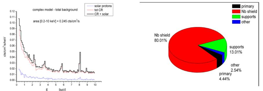
The spectrum of unvetted events (100 eV bin) with contributions from different input components highlighted, obtained with the detailed model.
